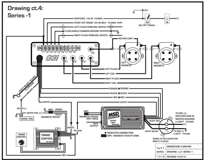
Left Magneto Retard Contacts are Trigger Source on Starting
