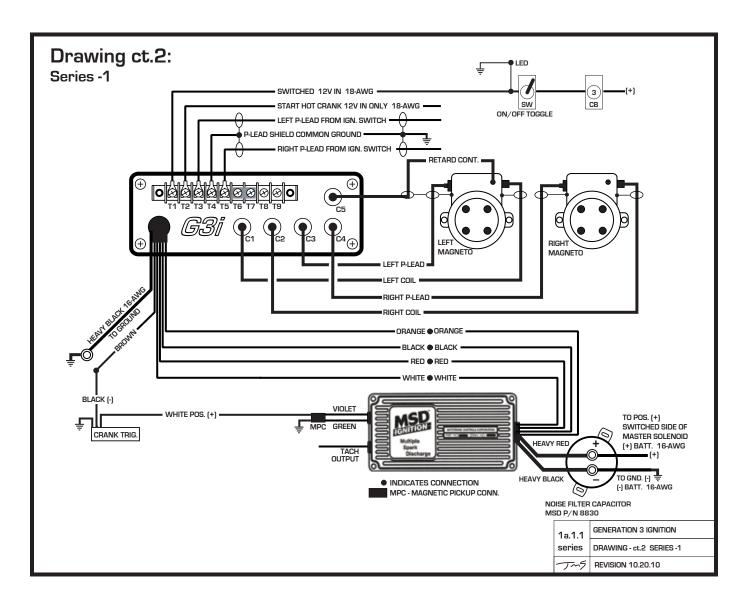
Left Magneto Retard Contacts are Trigger Source on Starting
